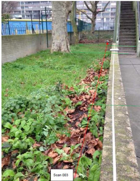
Fig 3 – By contrast scan lines within the planter areas showed significantly higher level of tree roots. This reinforces the need for their protection during all site works (demolition and construction)
