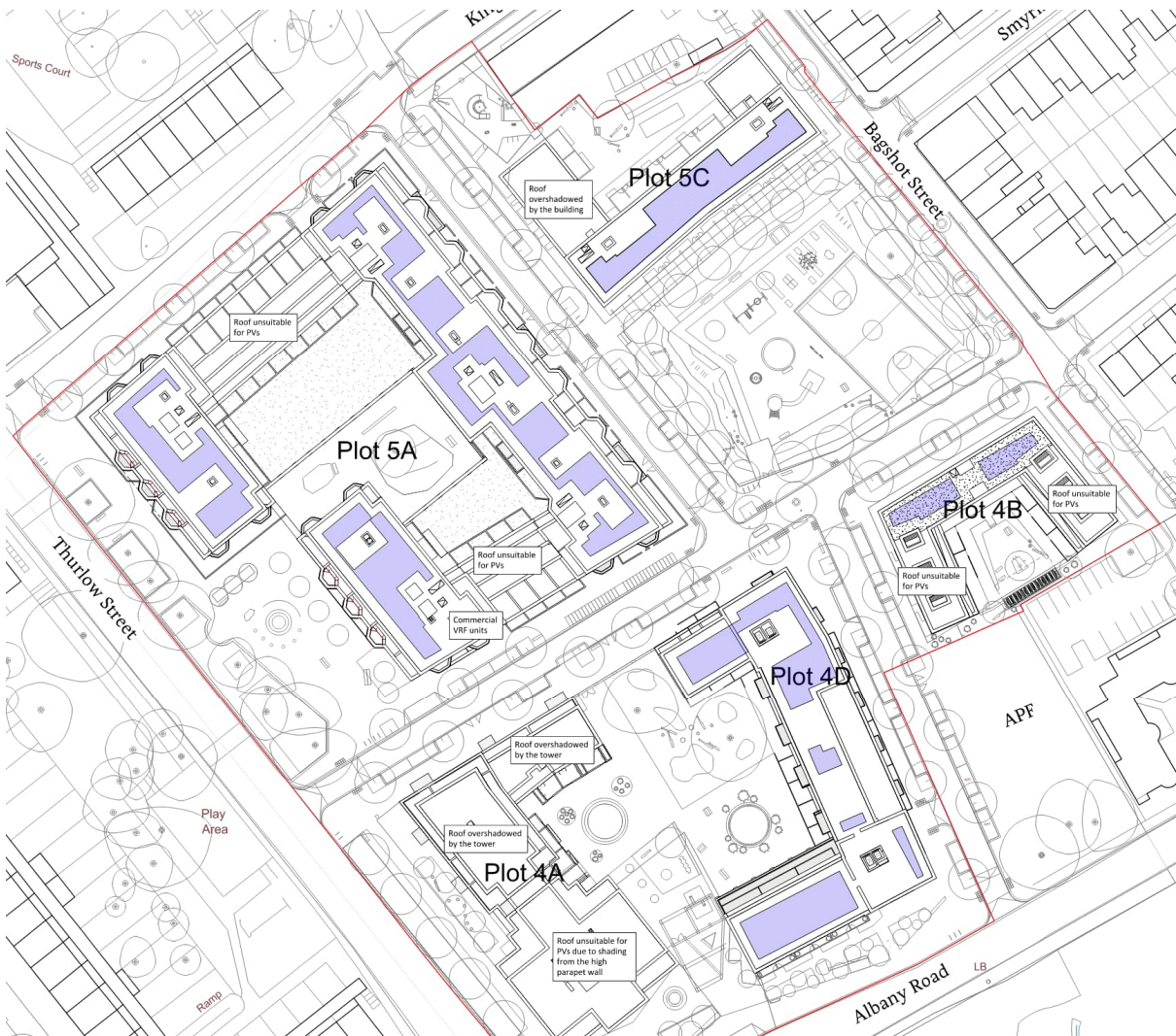
Figure 10: Solar PV installations areas shown in blue
