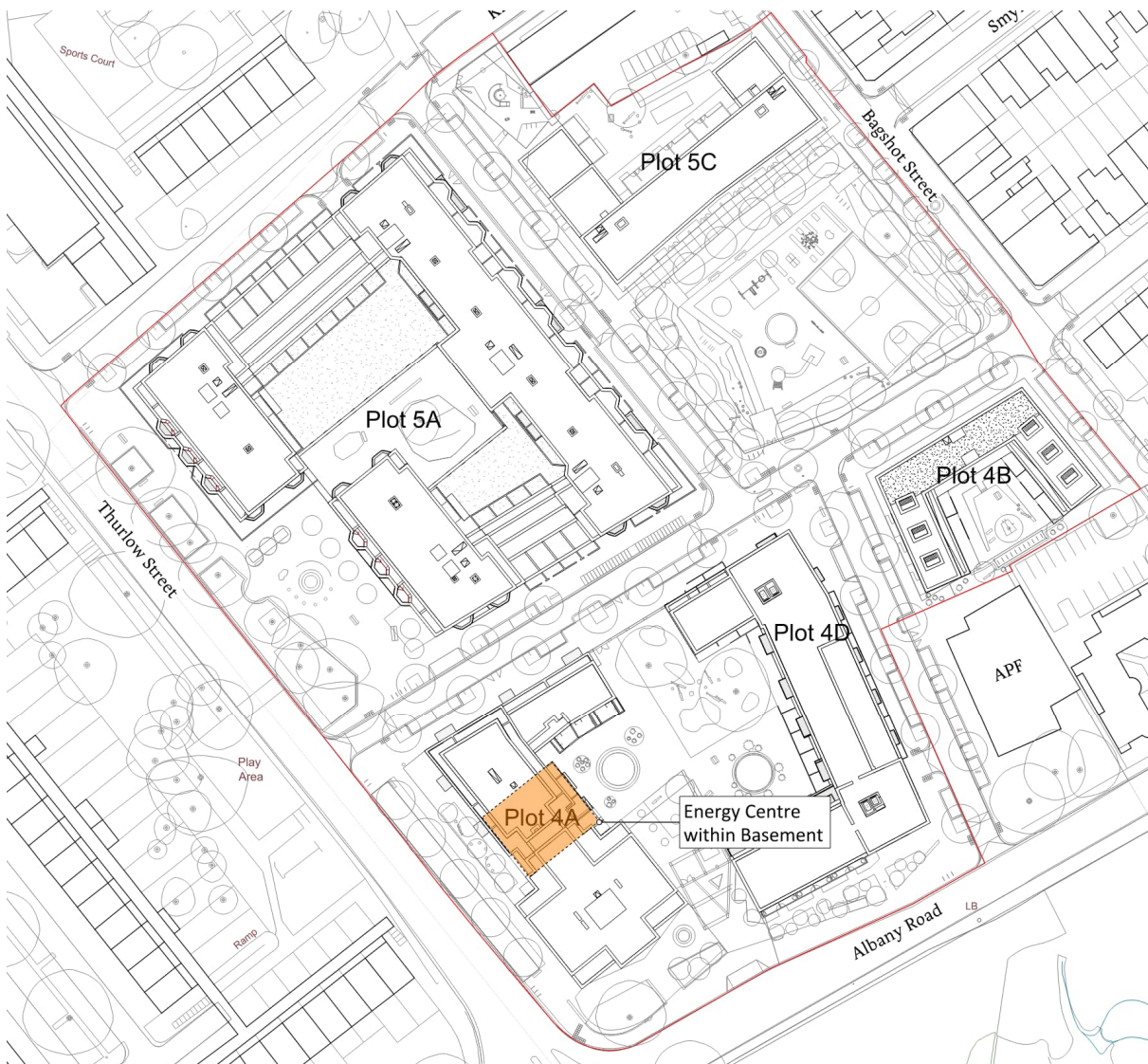
Figure 8: Proposed energy centre location for the site
