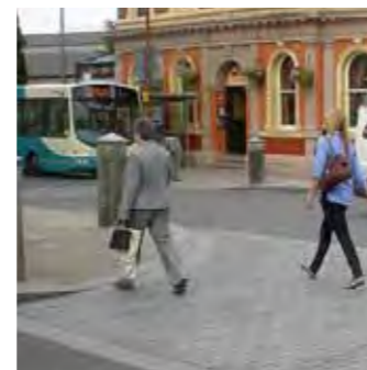
Crossing points to be paved with a consistent material to act as a visual cue to drivers to lower speed.
