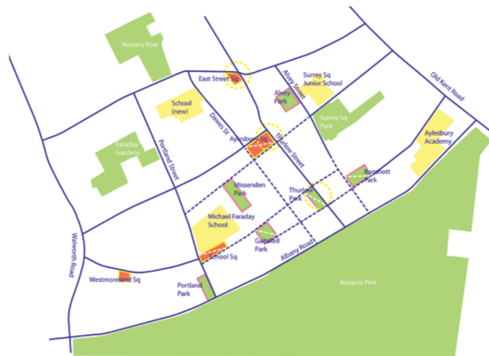
Fig 3.28 Early development of design teams approach to the Community Spines, using the areas of public open space to provide for changes in alignment along the routes
