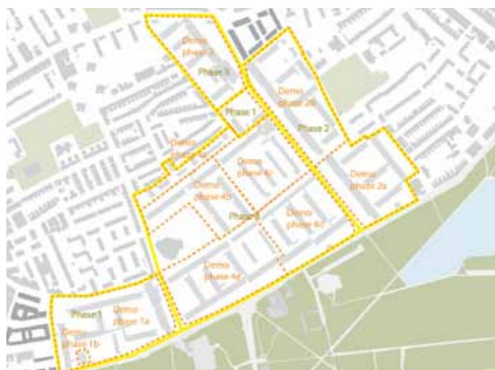
Fig 6.10 Phased demolition sites
