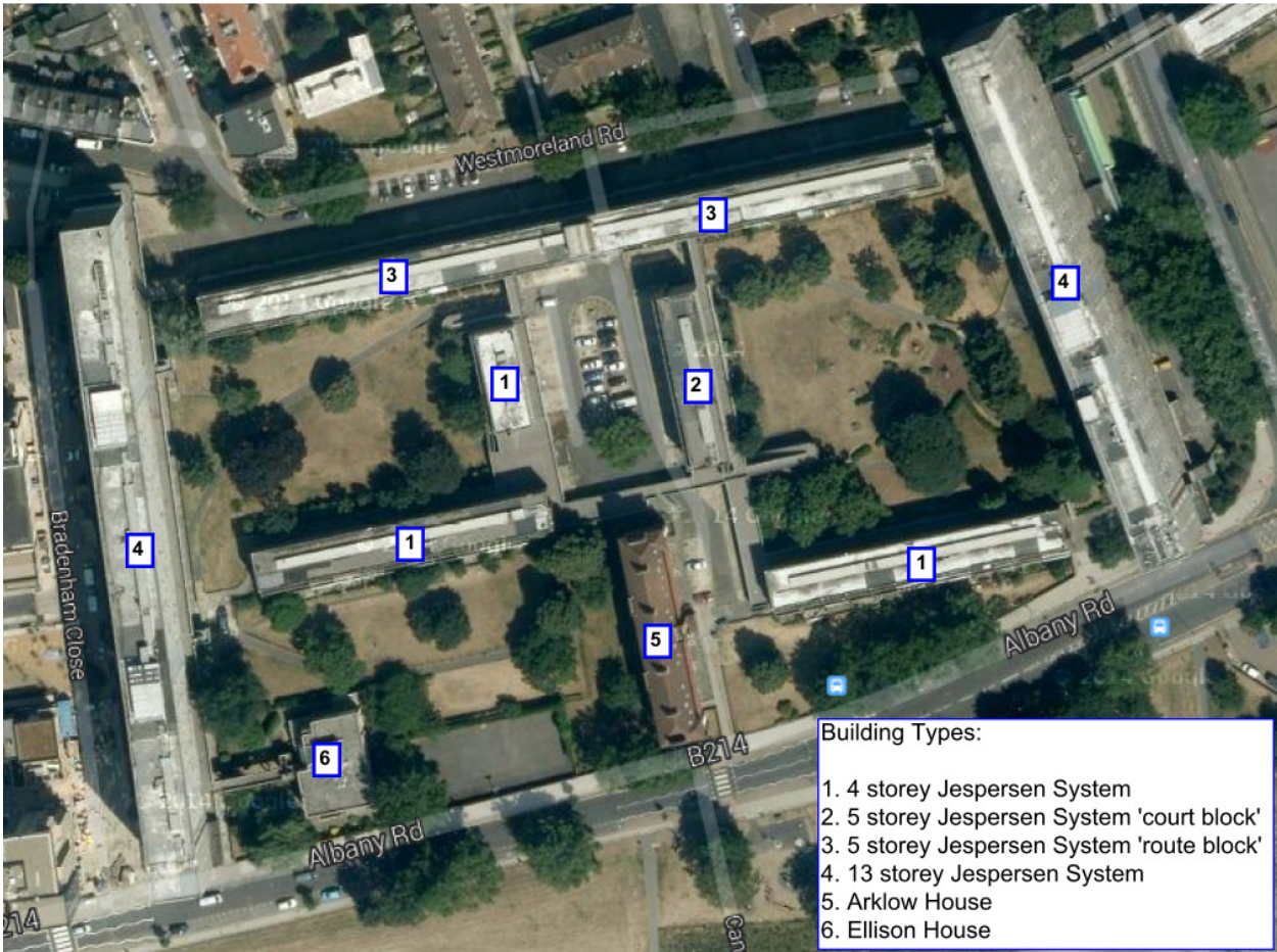
Figure 2: First Development Type building types.
