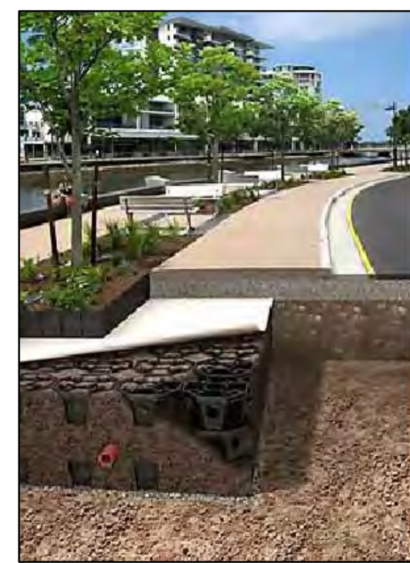
PROPOSED GEO-CELLULAR SOIL VAULT ASSEMBLY SVDs FEATURE TO PROVIDE SOURCE CONTROL OF LOCALISED SURFACE WATER RUNOFF AND TREATMENT PRIOR TO DISCHARGE TO PROPOSED SURFACE WATER SEWER OR WHERE APPLICABLE TWUL COMBINED SEWER NETWORK
